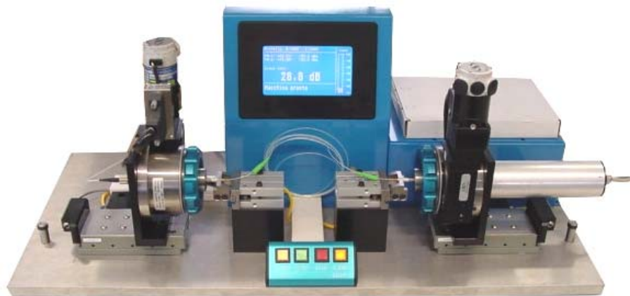
Figure 5: Measurement setup for the orientation of PM components using the cross polarizers method.
