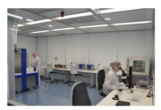
DIAMOND has created a **new ISO 7 cleanroom (class 10'000 according to FED STD 209E),** in order to supply products such as connector sets, pigtails, patchcords, adapters and mechanical parts that are cleaned and packaged in a controlled environment.
