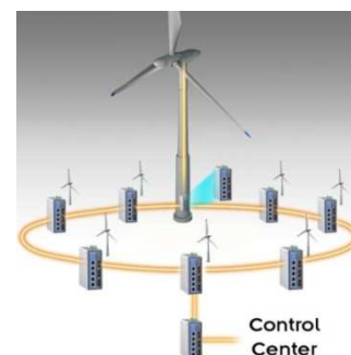
fig. 2 Fiber optic network for Wind Farms
