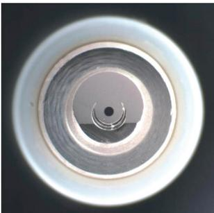
The primary function of a connector is to provide a repeatable low loss connection between optical fibers. High performance (low loss max. 0.1 dB) connectors must be able to minimize the factors, which lead to power loss. The primary drivers behind power loss are fiber-to-fiber eccentricity, contamination at the optical interface, and physical contact.
