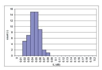
Based on our experience with SMF-28 fiber at 1550 nm an average IL of 0.045 dB on random mating can be expected, with a max value of 0.06 dB on 95% of the connections. At 1310 nm the IL values are higher due to the smaller mode field diameter. An average IL of 0.055 dB on random mating can be expected, with a max value of 0.10 dB on 95% of the connections.
