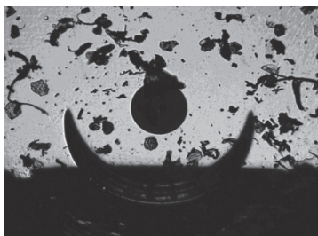
Contamination (Solid deposits)
