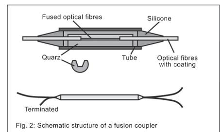
Fig. 2: Schematic structure of a fusion coupler
