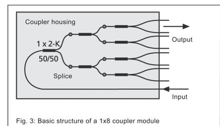
Fig. 3: Basic structure of a 1x8 coupler module
